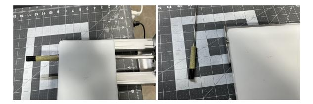
7. To release the extraction die the thumb lever must be pressed in, while this lever is depressed the knob of the extraction die can be pulled back. Only pull the die back as far as necessary to remove the mold. If the die is pulled back too far it is possible for the extractor to disassemble.
