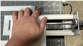
5. Repeatedly squeeze and release the extraction lever, this will force the extraction die into the core pressing it out of the mold. This process needs to be continued until the core is fully extracted from the mold. Failure to do this may result in breakage of the core.
