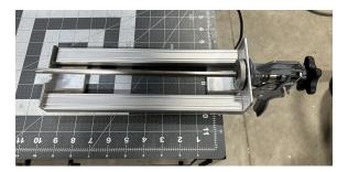
2. To release the extraction die the thumb lever must be pressed in, while this lever is depressed the knob of the extraction die can be pulled back. Only pull the die back as far as necessary to insert the mold. If the die is pulled back too far it is possible for the extractor to disassemble.
