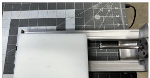
4. Pressing in on the thumb lever, the extraction die can now be slid forward against the top of the core. When the extraction process begins place one hand on top of the mold to provide support, failure to do this can result in damage to the extractor.
