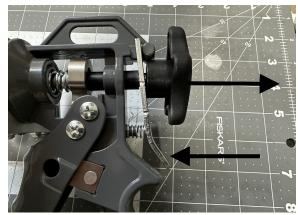
3. Insert the exposed skewer into the end of the extraction die, the core plug should be on the opposite end from the extraction die and should be aligned with the notch in the mold support.
